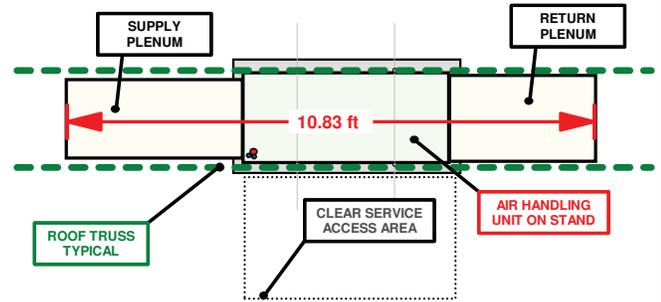
AIR HANDLER ON 24" TALL STAND REQUIRES 48" x 30" FOOTPRINT FOR BOTH SUPPLY AND RETURN AIR PLENUMS - PLENUMS ROUTE STRAIGHT UP BETWEEN TWO ROOF TRUSSES TO ATTIC ABOVE MAY ALSO ROUTE TO FLOOR TRUSS
